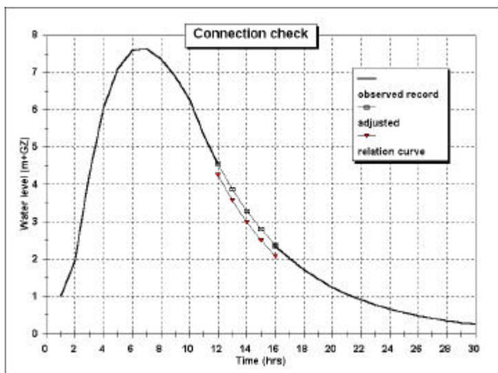
A relation curve based on the data of two series can be used to infill the missing data in the dependent variable of the relationship. The relation curve is used to calculate the missing value(s) at the station corresponding to the observed values at the adjacent station. An example is given in Figure 5.1.
