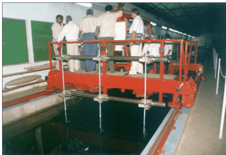
Figure.2: Close up of towing tank carriage
